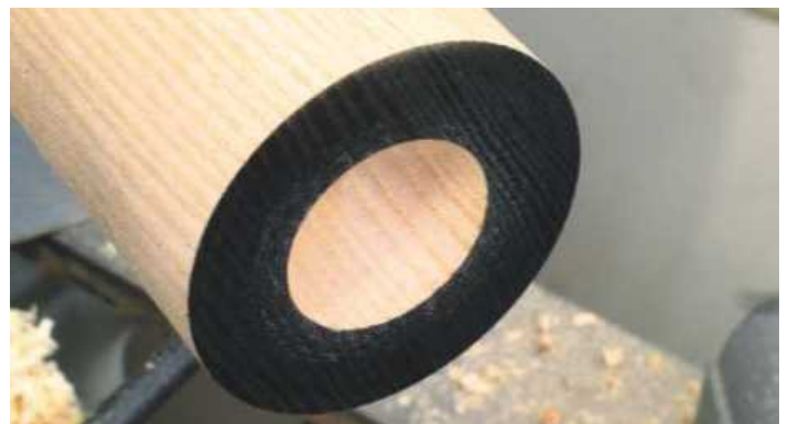
▲ Pic.16 If you decrease the depth of the cut as you get near your finished shape, you can achieve a pretty good finish. The denser the wood, the better the results you can expect
